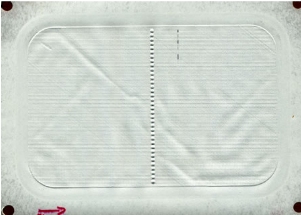
Figure 25. Scanned-in images of fouled membranes from a desktop scanner. The membranes are: (a) H. pygmaea shearing run, (b) post-MF (microfiltered) run, (c) post-UF (ultrafiltered) run, and (d) a control coupon where the membrane was run with only sodium chloride solution (NaCl run).
