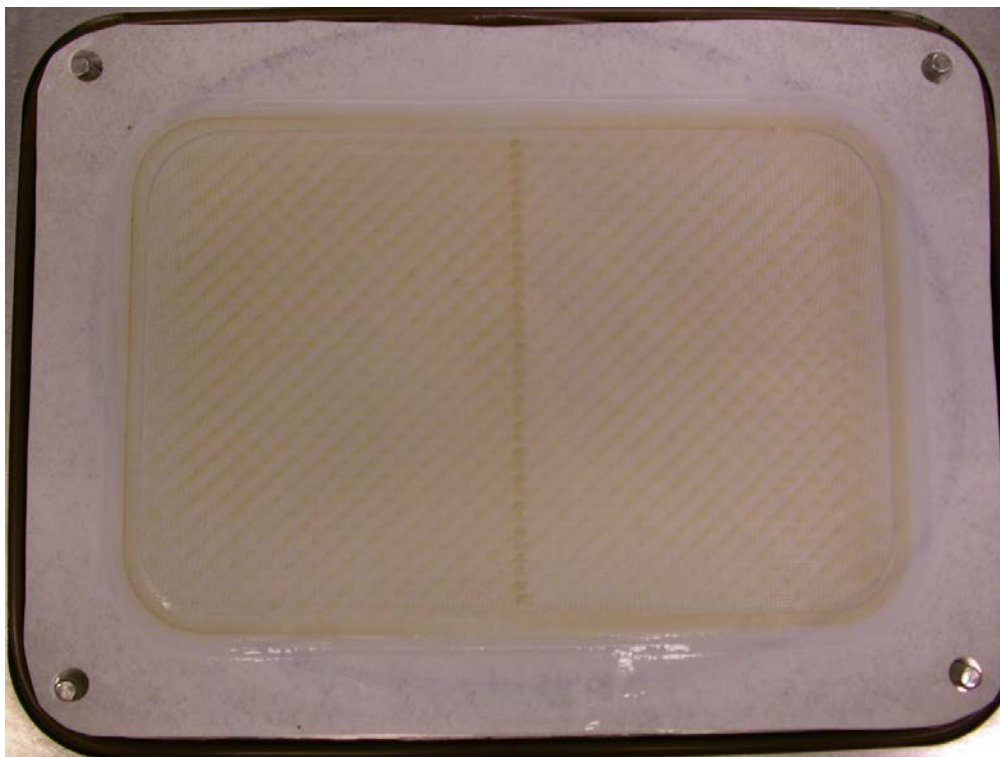
Figure 17. Photograph of the RO membrane coupon after a 4-day test with the sample throughput protocol.
