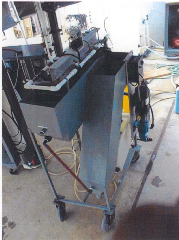
Figure 4-10: Coagulation/Flocculation/Sedimentation Unit Setup
