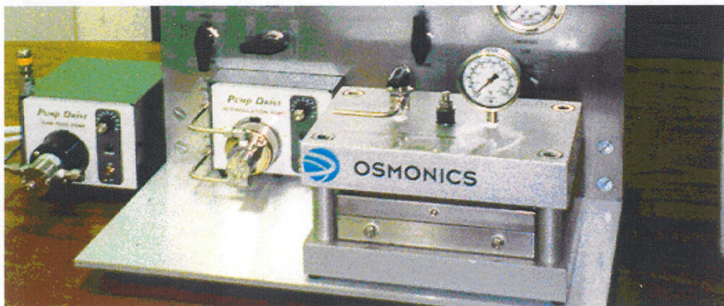
Figure 4-7: Osmonics Flat Sheet Sepa® Membrane Cell System
