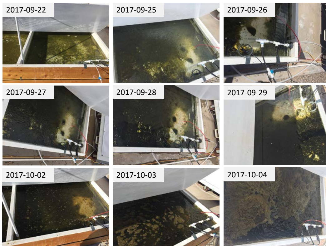
Figure 27.—Less green algae in the photobioreactor after the nutrient regulations.
