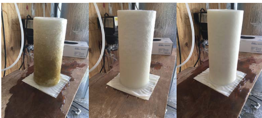
Figure 32.—Appearance of cartridge filters after use (pore sizes: 10, 10, and 5 \mu\text{m} ).
