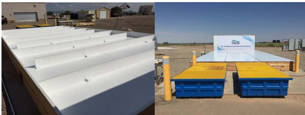
Figure 8.—1,500-gallon photobioreactor (left: uncovered, right: covered) and two 250-gallon water storage tanks (right, blue-yellow tanks).
