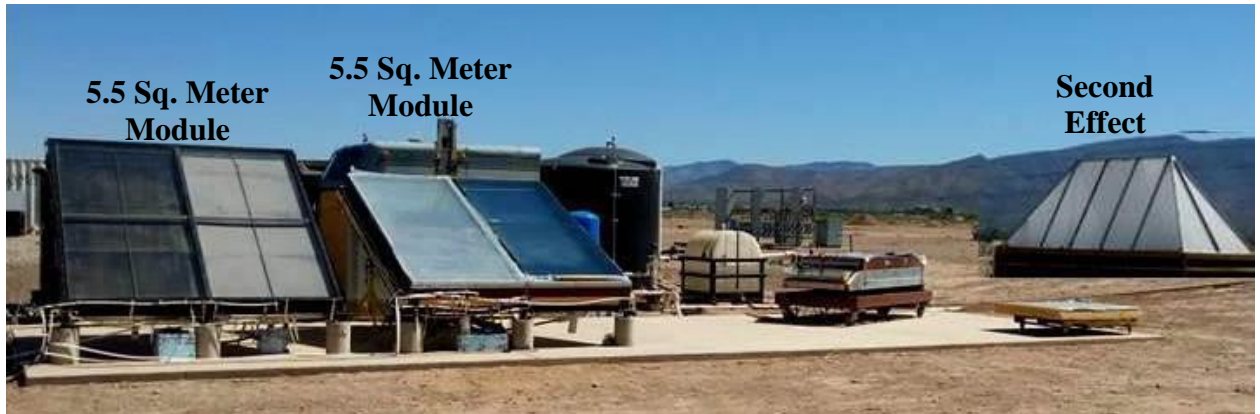
Figure 2. Two 5.5 square meter modules at left and the 12 square meter by 1 meter deep Second Effect at right.
