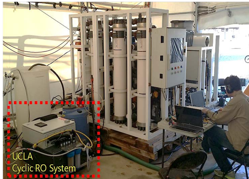
Figure 13. Deployment of the UCLA CRO system at the Naval Facilities Engineering Command's Seawater Desalination Test Facility (NAVFAC SDTF) in Naval Base Ventura County.
