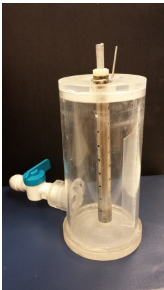
Figure 2. Photograph of the custom-designed, plexi-glass electrochemical cell employed in all experiments.
