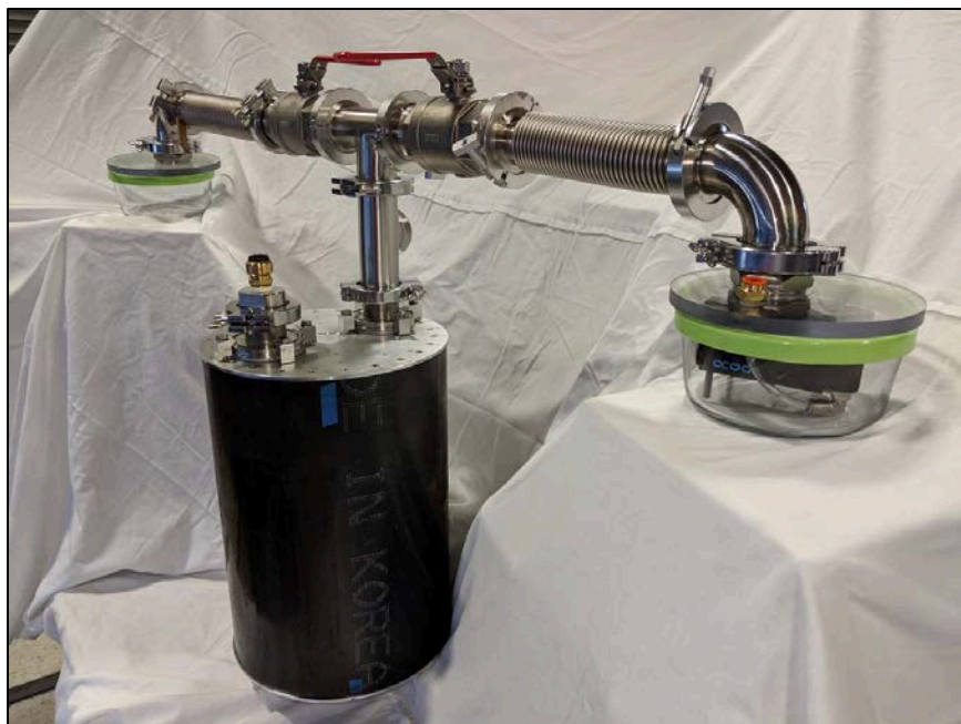
Figure 9. Completed proof-of-concept adsorbent bed with evaporator and condenser
