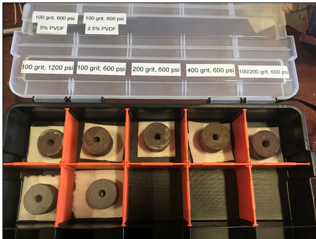
Figure 4. Annular adsorbent samples fabricated for permeability testing
