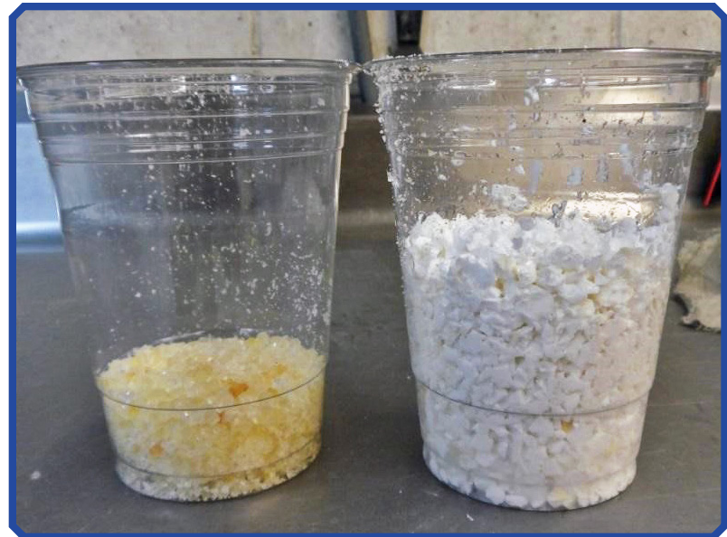
Ground-up hydrophilic waterstop before water was added (left) and after water was added (right). The cups contained the same volume of waterstop prior to activation.
