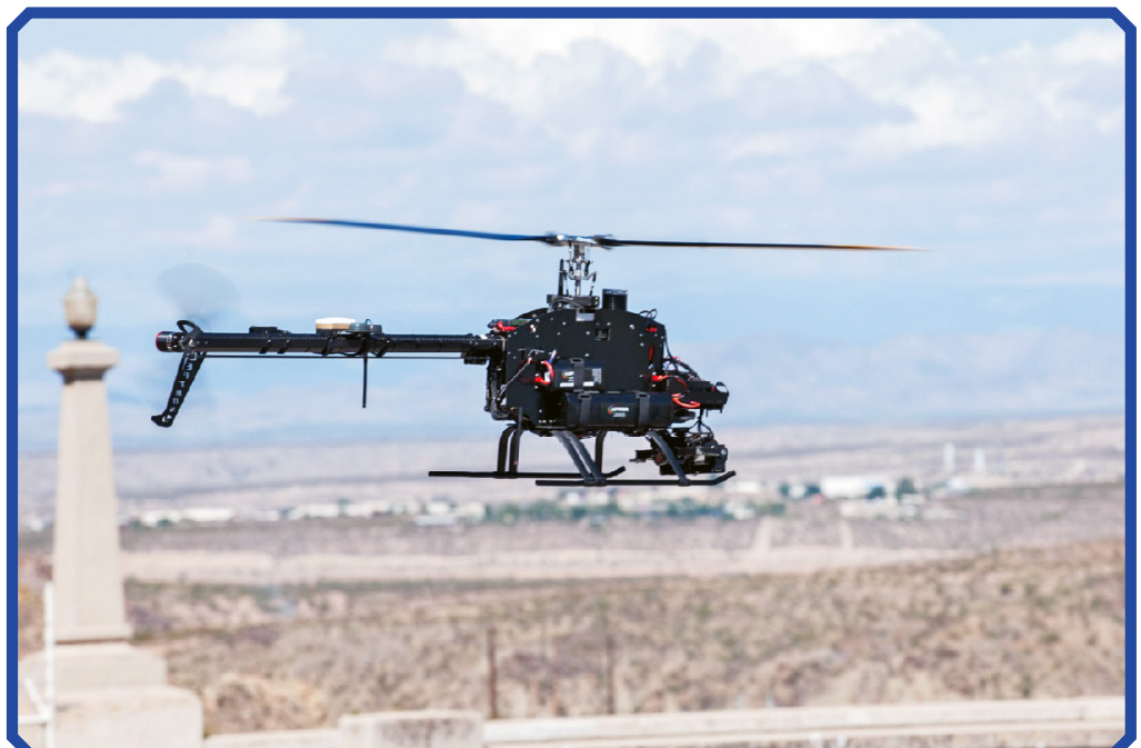
Lepton Avenger E Model UAS at Elephant Butte Dam, New Mexico. Note sensor gimbal at the front of the airframe.
