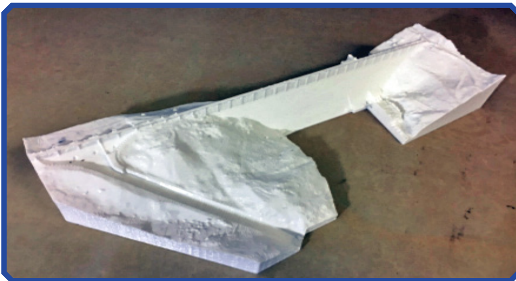
A 3D print of the photogrammetric model of Elephant Butte Dam, New Mexico.
