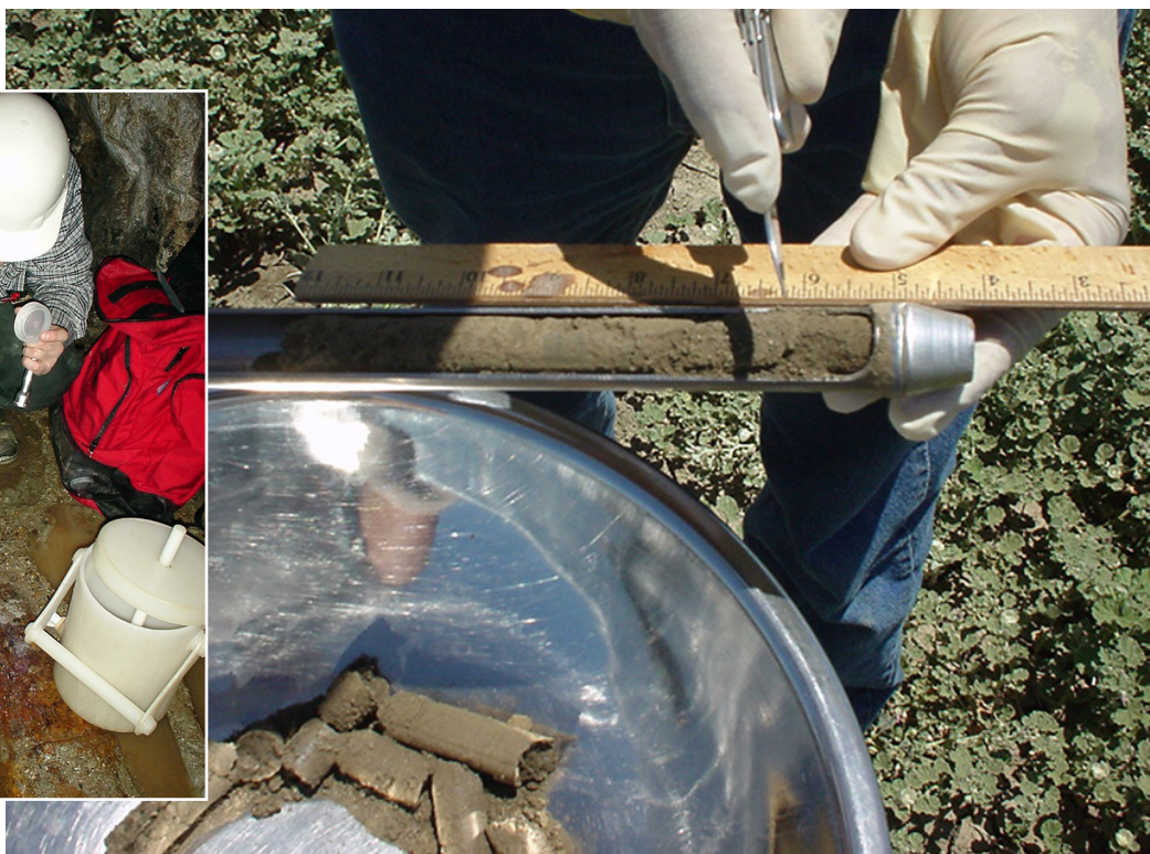
Soil core collection at a former airfield near the Delta Mendota Canal.
