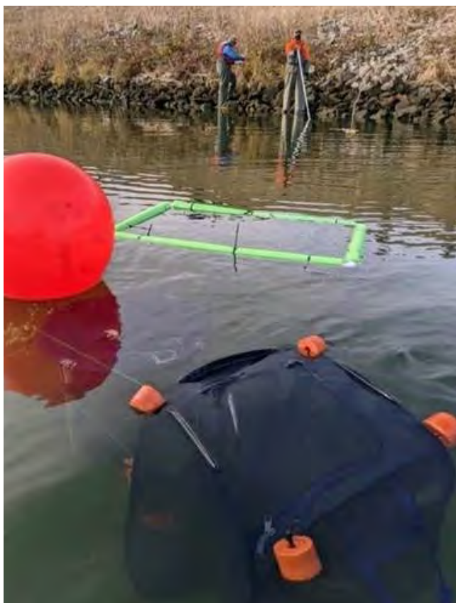
Live pen experiment at Shag Slough, San Francisco Bay-Delta, California, to evaluate distance and conditions at which environmental DNA from fish species can be detected.
