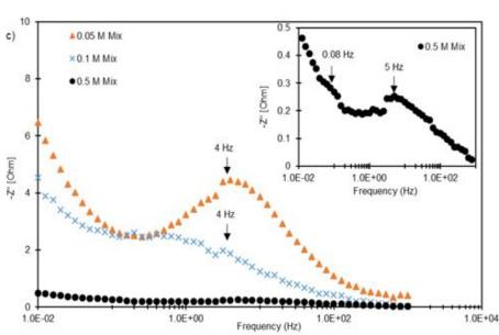
Bode plots for different ionic strengths solutions of CR671. (a) NaCl, (b) CaCl<sub>2</sub>, (c) Mixed NaCl + CaCl<sub>2</sub> (Na<sup>+</sup>/Ca<sup>2+</sup>, 7.2:1).
