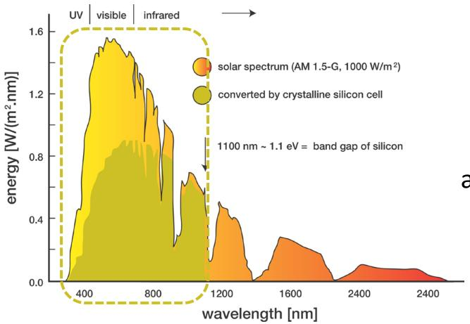
Silicon PV panels convert ~20% of the available solar power to electricity
