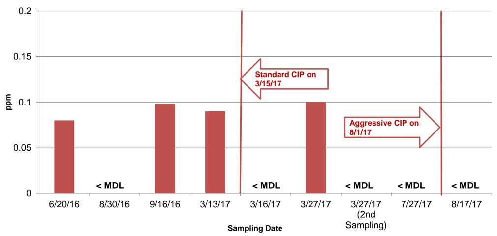
Feed TOC = 5 - 10 ppm Target Permeate TOC < 0.5 ppm MDL (Method Detection Limit) = 0.0331 ppm
