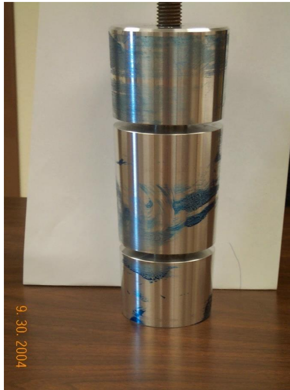
Photo 6.—Wicket gate shear pin.
