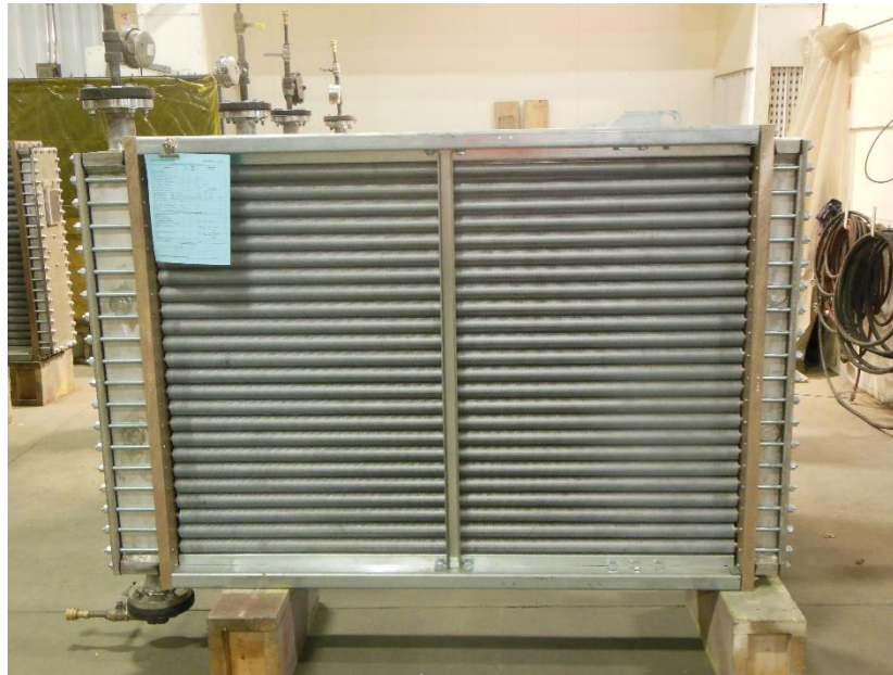
Photo 15.—Generator air cooler.
