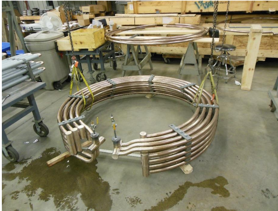
Photo 16.—Cooling coil for turbine bearing.
