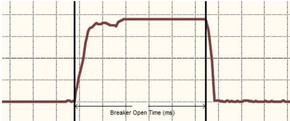
Figure 2-2. Breaker close-open-close timing
