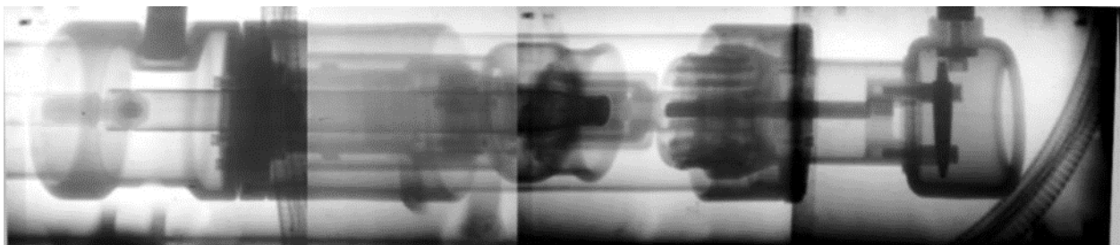
Figure 8-4. Radiographic image of a circuit breaker
