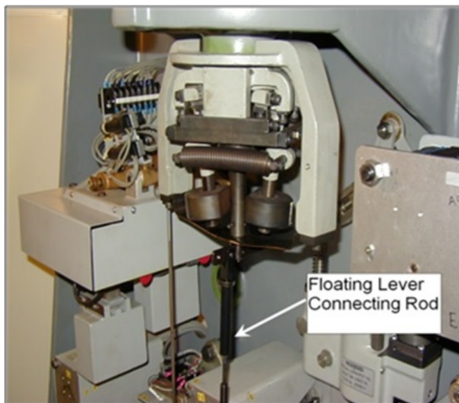
Photograph 18. Woodward ballhead and floating lever connecting rod
