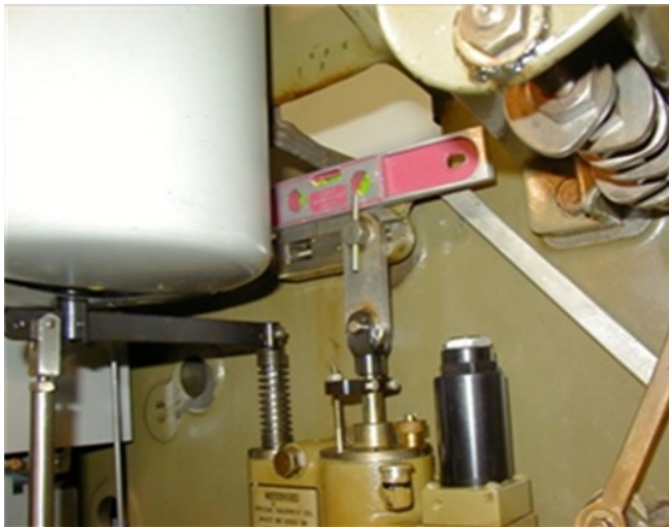
Photograph 1. Leveling compensating crank
