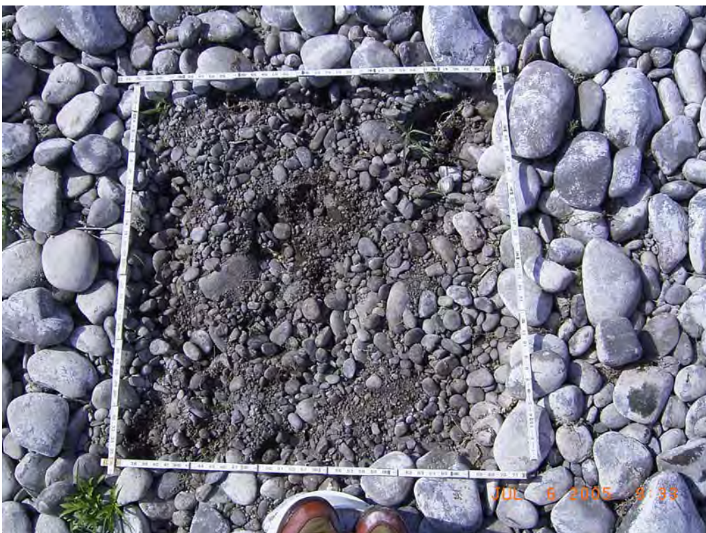
Figure 11. Photograph of the sampling area after removal of the surface material
