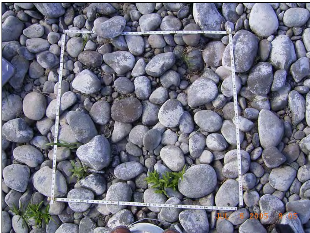
Figure 10. Photograph of the sampling area prior to the removal of the surface material
