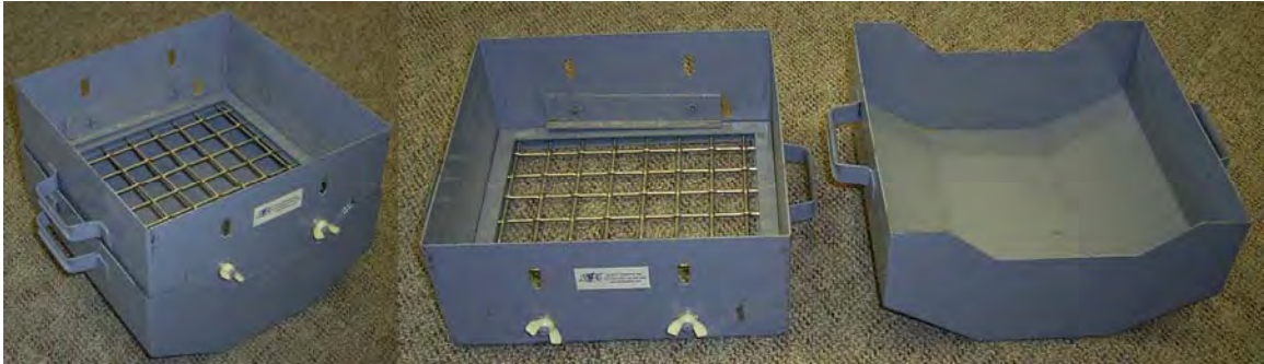
Figure 12. Field sieve used for fractions finer than 64 mm. The 32-mm screen is shown
