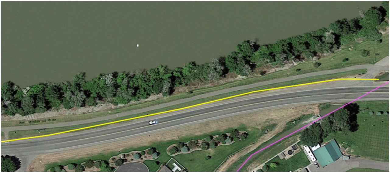
Figure 2. Representative example of the estimated location of the existing pipeline (in yellow) between Fir Street and the paved pathway
