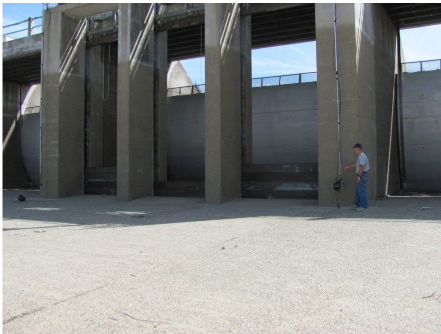
Figure 2. Picture of DTX split-beam transducer prior to reservoir levels rising to spillway elevations. The ROS rotator can be seen to the left of the sonar head, which was attached via a custom fabricated aluminum plate. In the lower picture, both units can be seen hanging from the safety rail at the top of the gate structure, one on either side of the gates, used for spilling during the study period.
