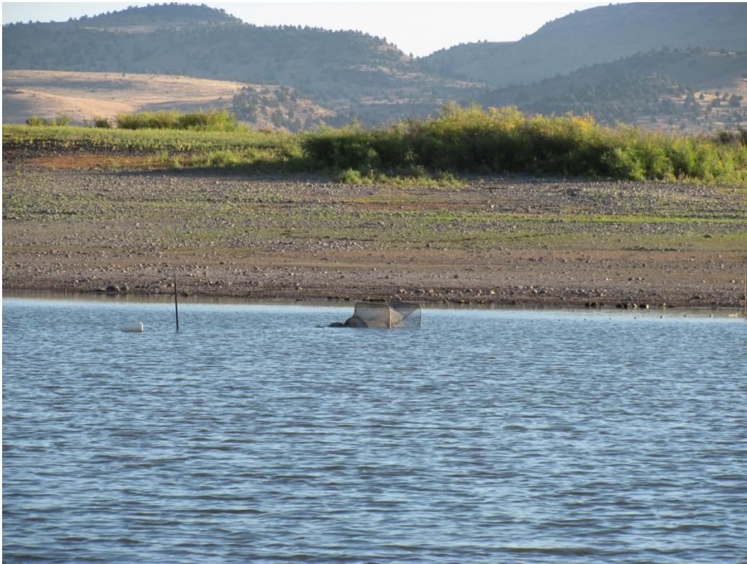
Figure 11. Typical fyke net set in Beulah Reservoir with lead line running to shore.
