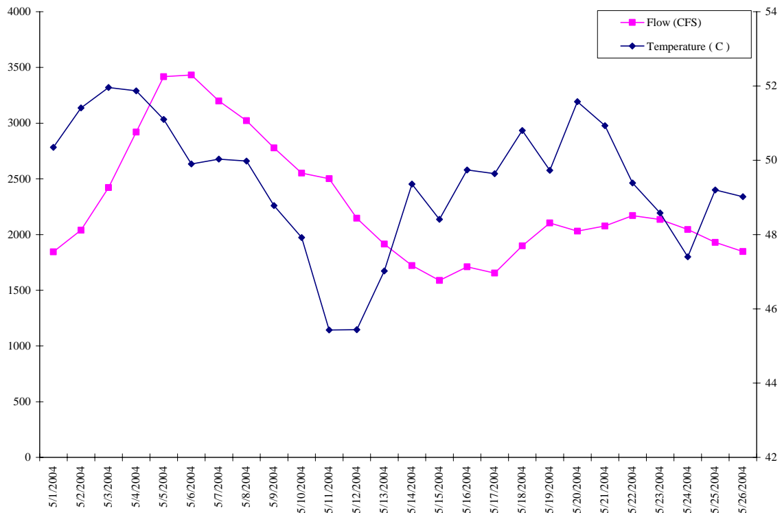
Figure 2. Mean daily water temperature (degrees Fahrenheit) and stream flow ( \text{ft}^3/\text{s} ) of the Middle Fork Boise River at Twin Springs gauging station.
