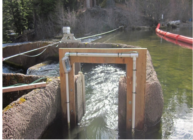
Antenna at exit of pool-and-weir fish ladder
