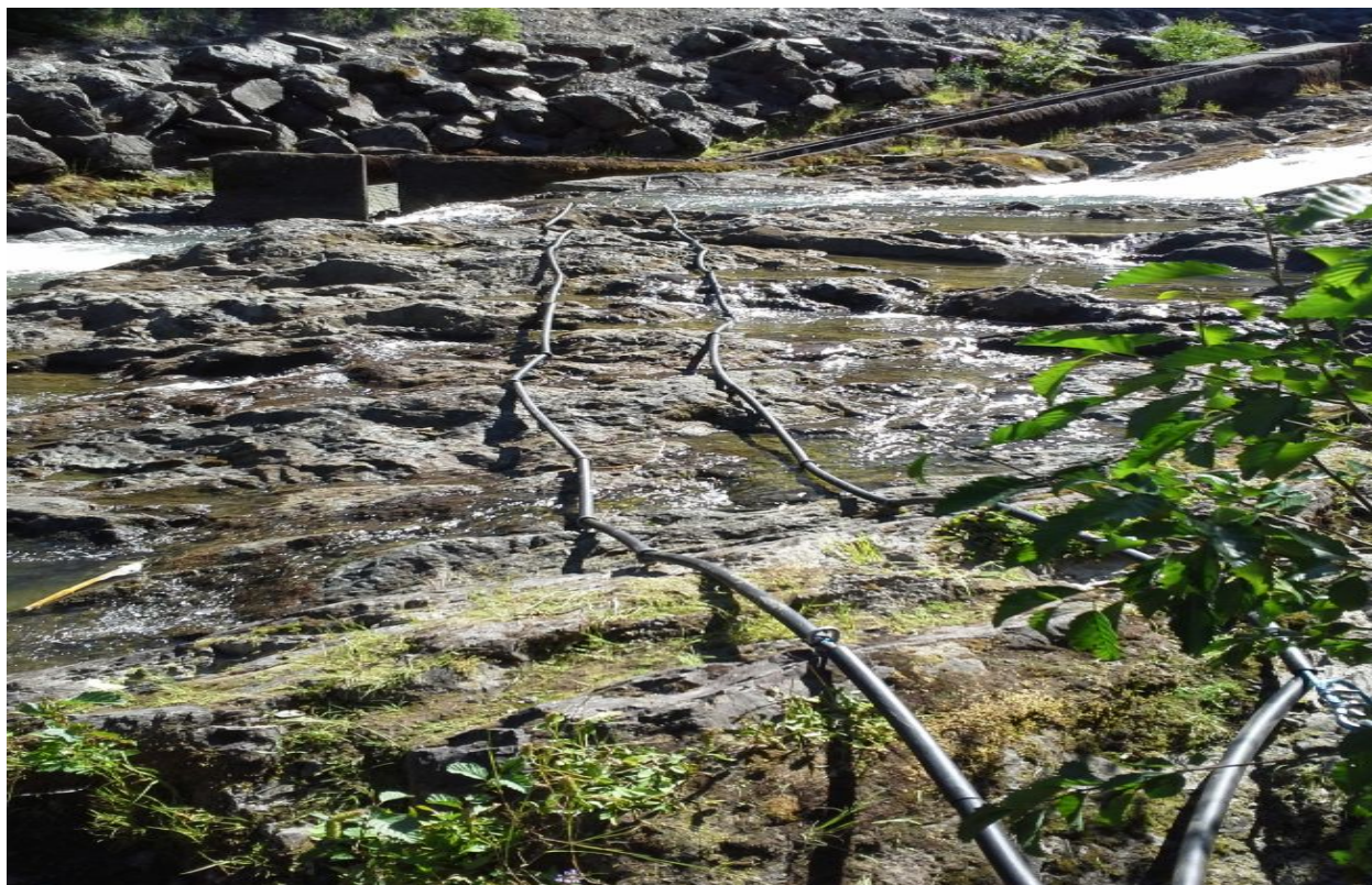
Figure 2. Reinstalled "beaver resistant" lower spillway antenna (July 9, 2014)
