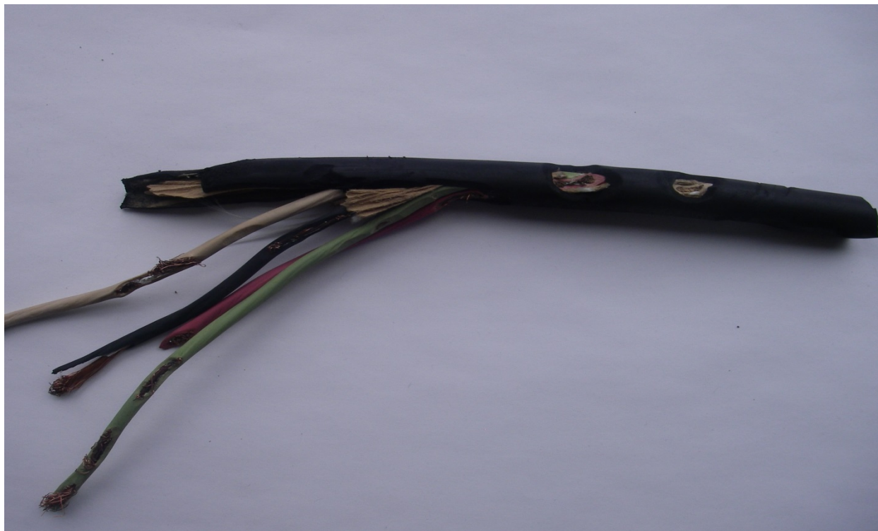
Figure 1. Damage inflicted on the lower spillway antenna by a suspected beaver in May 2014.
