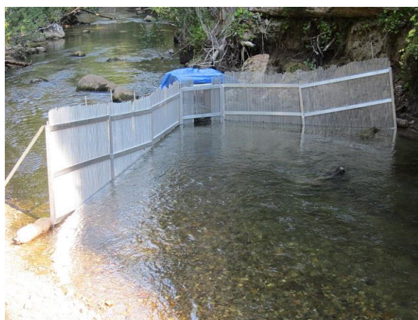
Completed picket-weir and box trap
