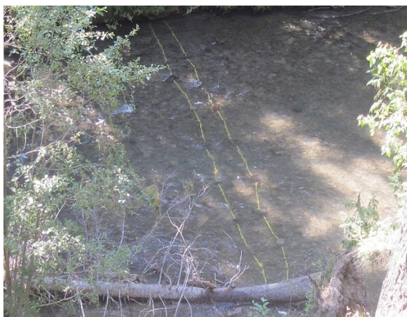
NF Tieton River PIT tag detection antenna
