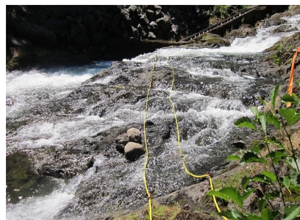
Lower spillway PIT tag detection antenna
