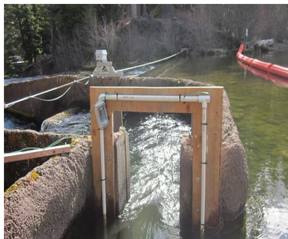
Upper ladder PIT tag detection antenna
