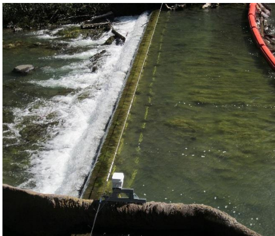
Upper spillway PIT tag detection antenna
