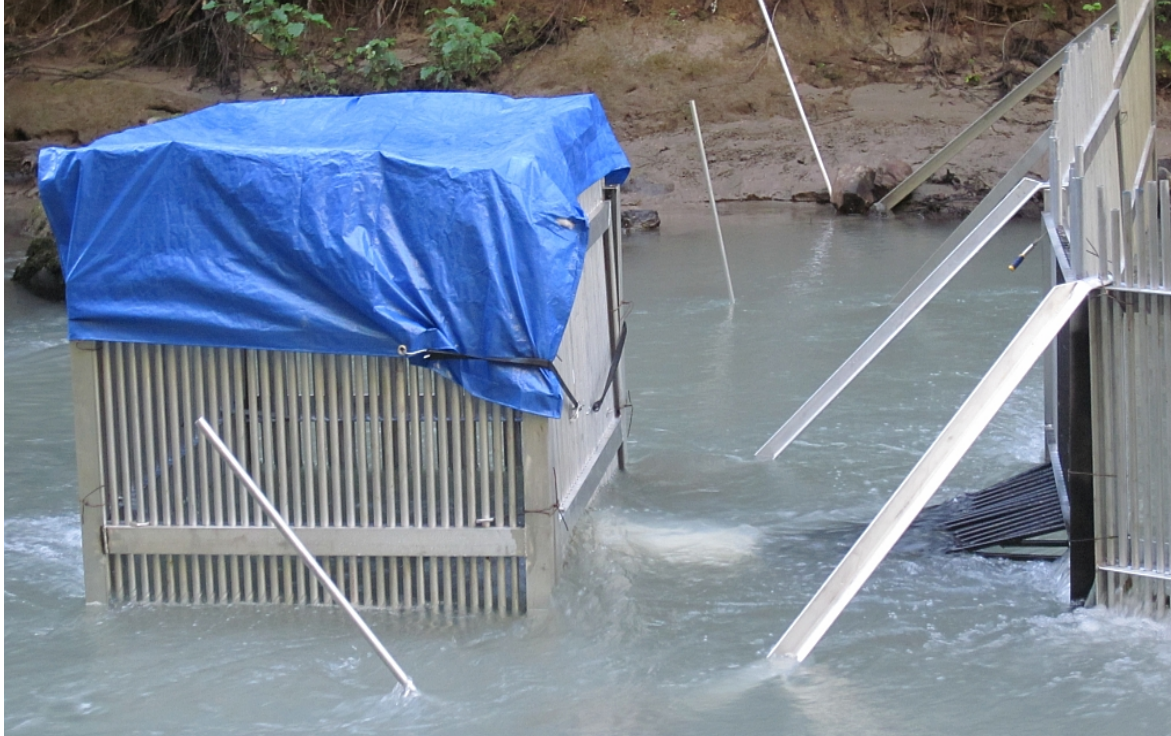
Figure 8. The modified configuration of the trap used in 2013. Note the modified entrance leading to the PVC pipe extending into the trap. The trap itself sits about five feet from the entrance.
