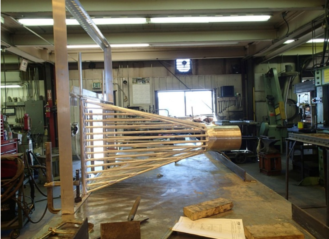
Figure 7. Modification to the entrance of the 2013 trap in WDFW's screen shop
