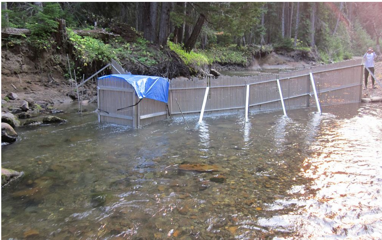
Figure 6. The picket-weir box trap use in 2012 on the North Fork Tieton River
