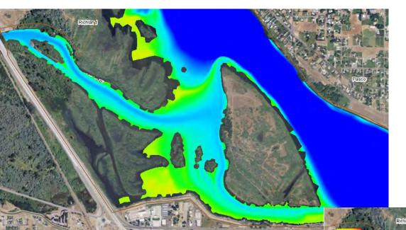
Varying causeway breach sizes and configurations
