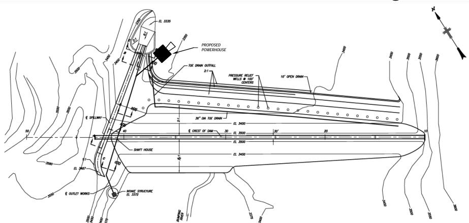
• Configuration identical to 1985 design for large Bumping Reservoir with crest elevation 70 feet lower.
