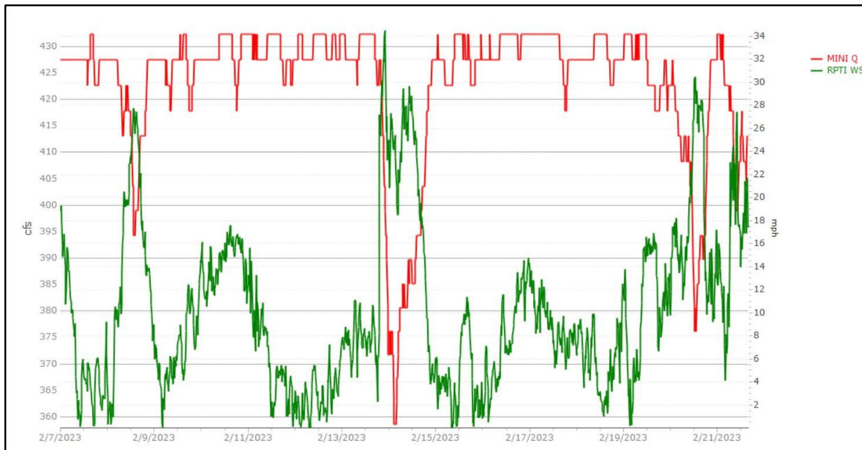
Figure 12. Figure showing data correlation between reduced streamflow gage readings (shown in red, "MINI Q") and increased wind speed data recorded at the Rupert weather station (shown in green, "RPTI WS"). Dips in streamflow readings occur when sustained wind causes water stacking in the area between Minidoka Dam and the downstream gage. Data shown are for February 7-22, 2023.
