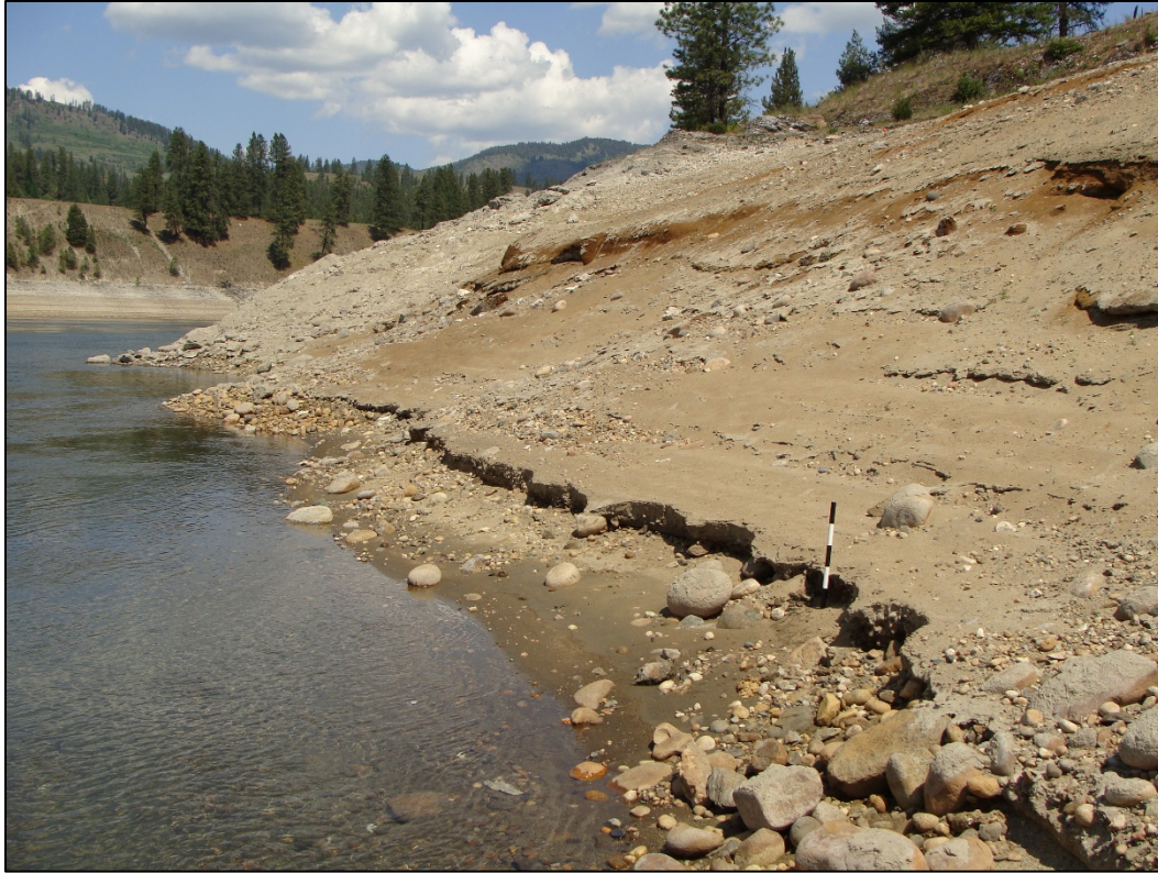
Figure 3-1. The material at the Marble Beach stabilization site consists of gravelly sandy loam with rock outcropping and cobbles.
