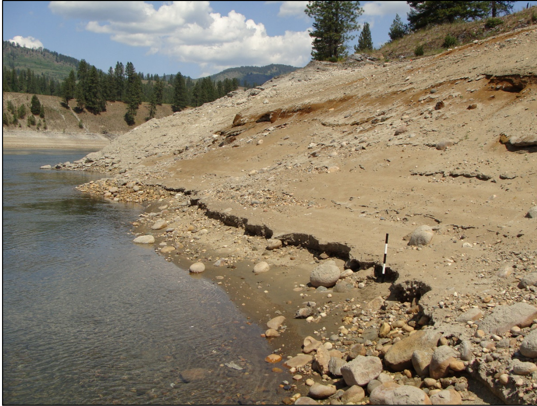
Figure 3-1. The material at the Marble Beach stabilization site consisting of gravelly sandy loam with rock and outcropping and cobbles.
