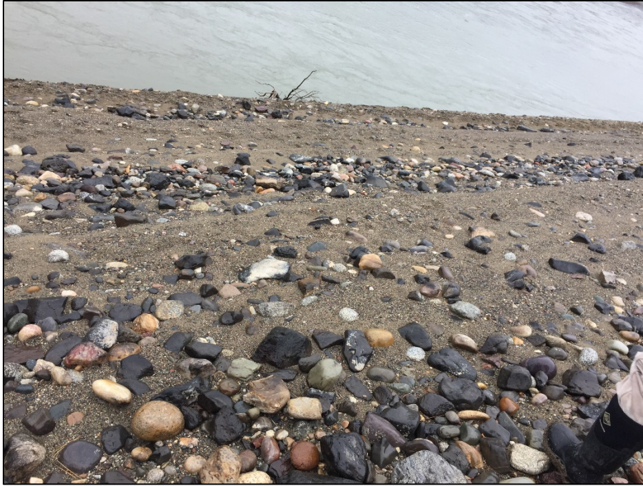
Figure 6. The material at the terrace is composed of alluvial material consisting of sand and gravel with cobbles
