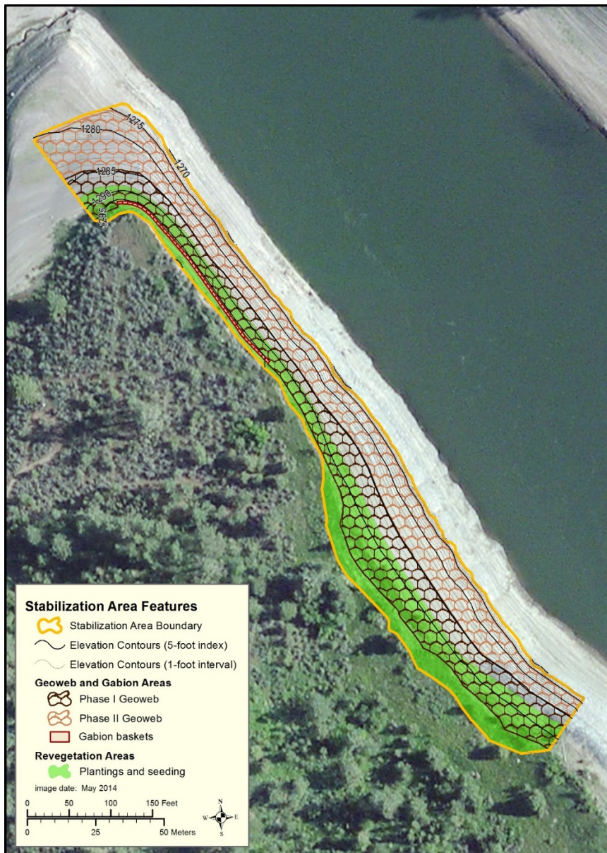
Figure 3. Cayuse Cove slope stabilization Phases I and II
