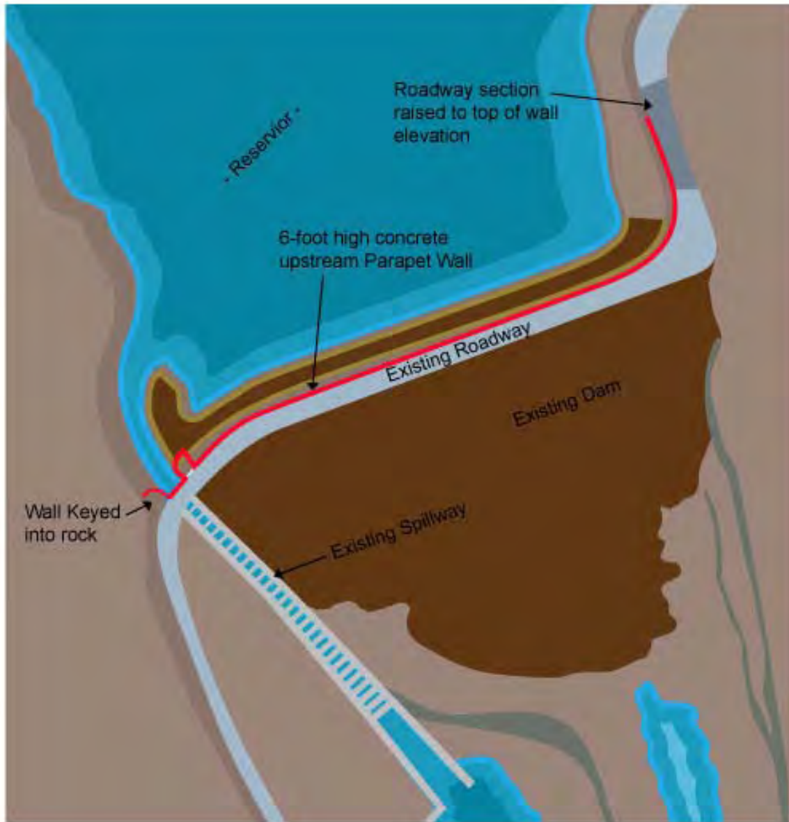
Figure 1. Alternative B, concrete parapet wall and modified spillway.
