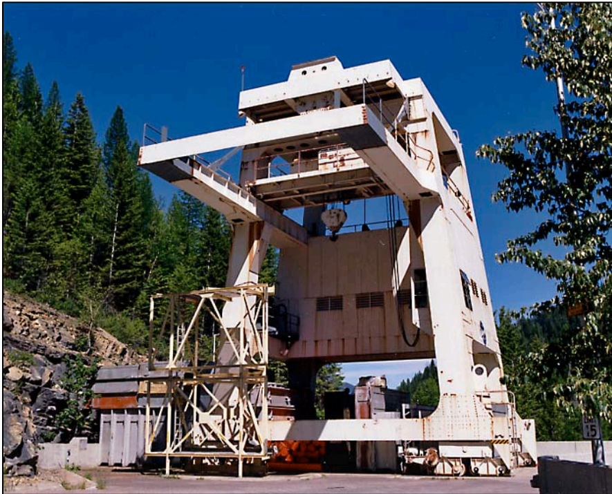
Photograph 1-3. Forebay gantry crane at Hungry Horse Dam
