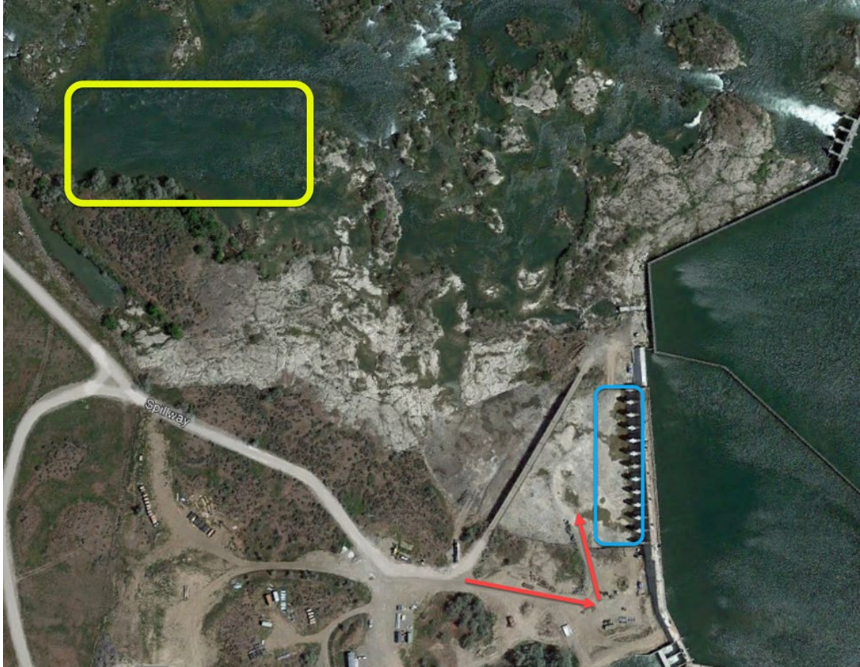
Figure 8. Aerial imagery of the seasonally-dewatered action area during previous construction activities in 2014, showing the location of previous temporary access road (red arrow), proposed construction area (blue box), and occupied Snake River physa habitat (yellow box)
