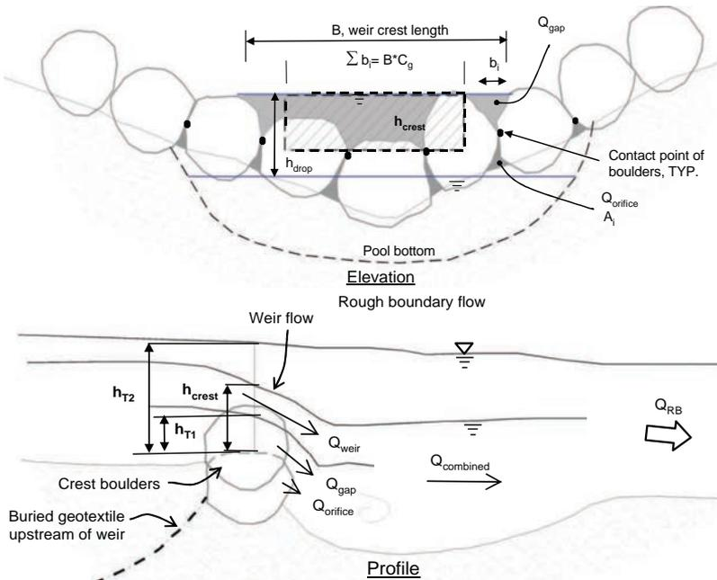
Figure 1. Elevation and profile of four-mode hydraulic model at rock vortex weirs.
