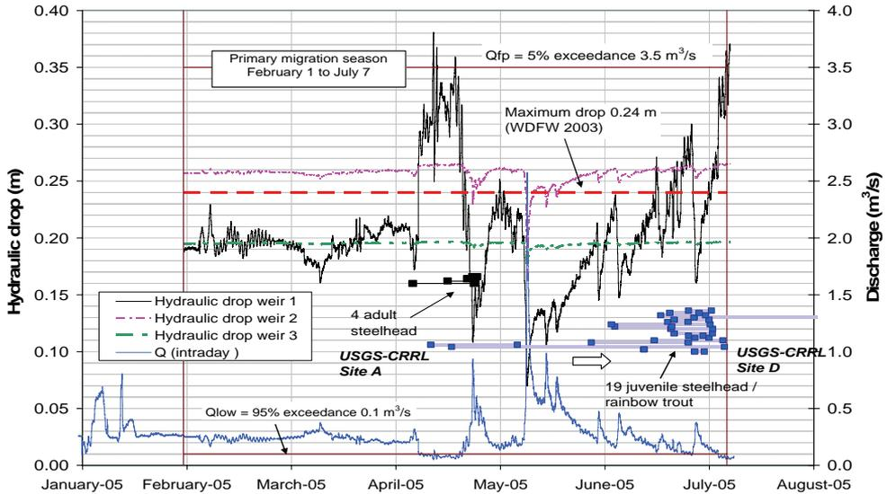
Figure 3. Comparison of fish movement from USGS-CRRL to calibrated hydraulic model of drop at rock vortex weirs at Lower Stokes during 2005 primary migration season. Horizontal bars for fish movement from left to right indicate detection time 3 km downstream (Site A or Site B) to detection time upstream, about 100 m upstream of the rock vortex weirs at Lower Stokes (Site D).
