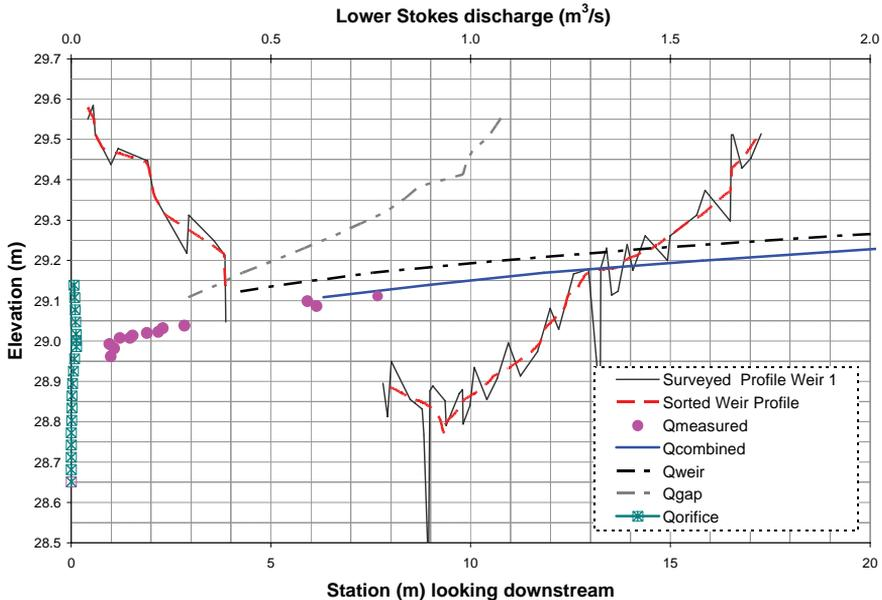
Figure 2. Hydraulic model at Lower Stokes, weir 1. Cross section compared to stage-discharge relations for the hydraulic model. Axes for cross section station and discharge on bottom and top, respectively. Individual flow modes ( $Q_{\text{orifice}}$ ,  $Q_{\text{gap}}$ , and  $Q_{\text{weir}}$ ) and total modeled flow ( $Q_{\text{combined}}$ ) compared to measured stage versus discharge. Relative flow contributions of flow modes versus stage shown.
