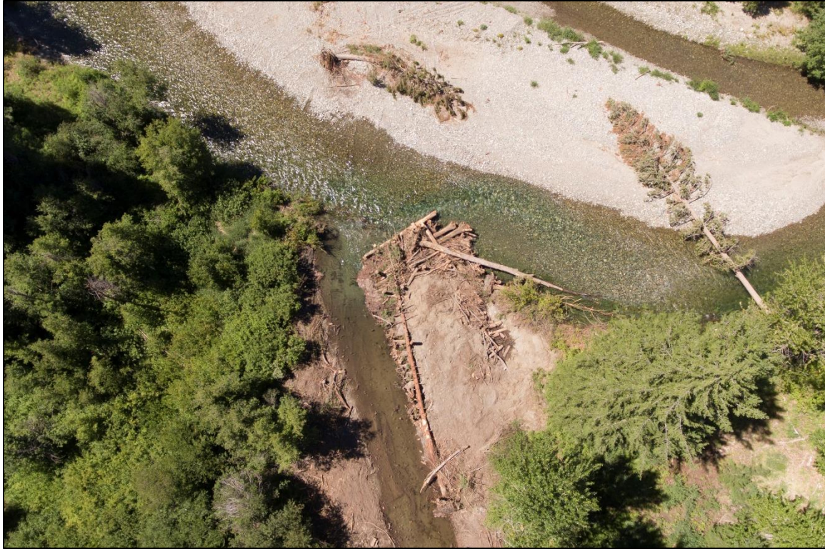
Figure 36. Excavating pools and installing log jams increases habitat suitability for spring Chinook and steelhead. Photo is of log jam on the Chewuch River installed as part of enhancement actions at the Chewuch RM 10 site.
