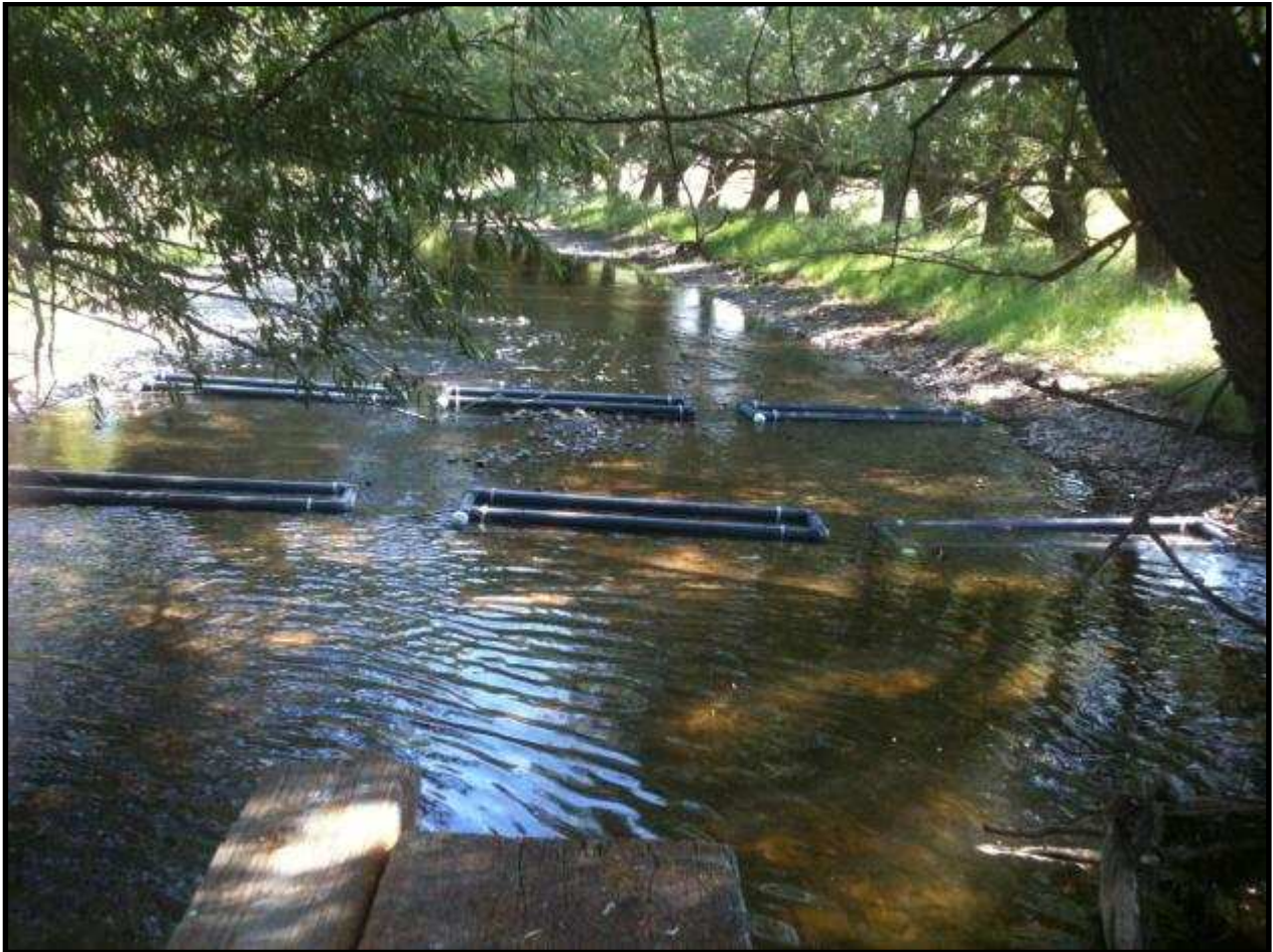
Fig. 5: Antenna configuration of the PIT tag interrogation system installed at Yeargain Bridge. Antennas were spaced approximately two feet apart to maximize coverage of the waterway.
