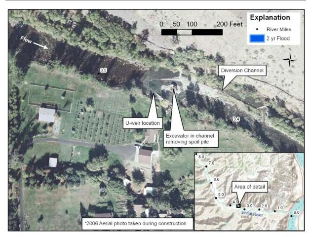
Figure 32. Bridge-to-Bridge Phase I (Whitehall Weir) site map.
