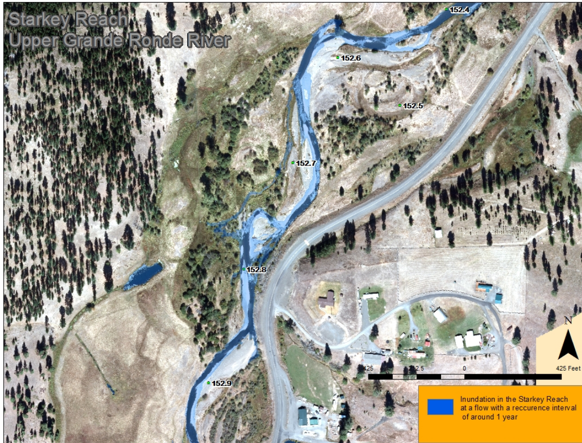
Figure 12. Activation of an intermittent side channel within the Starkey reach during a flow with a return interval of approximately 1 year.
