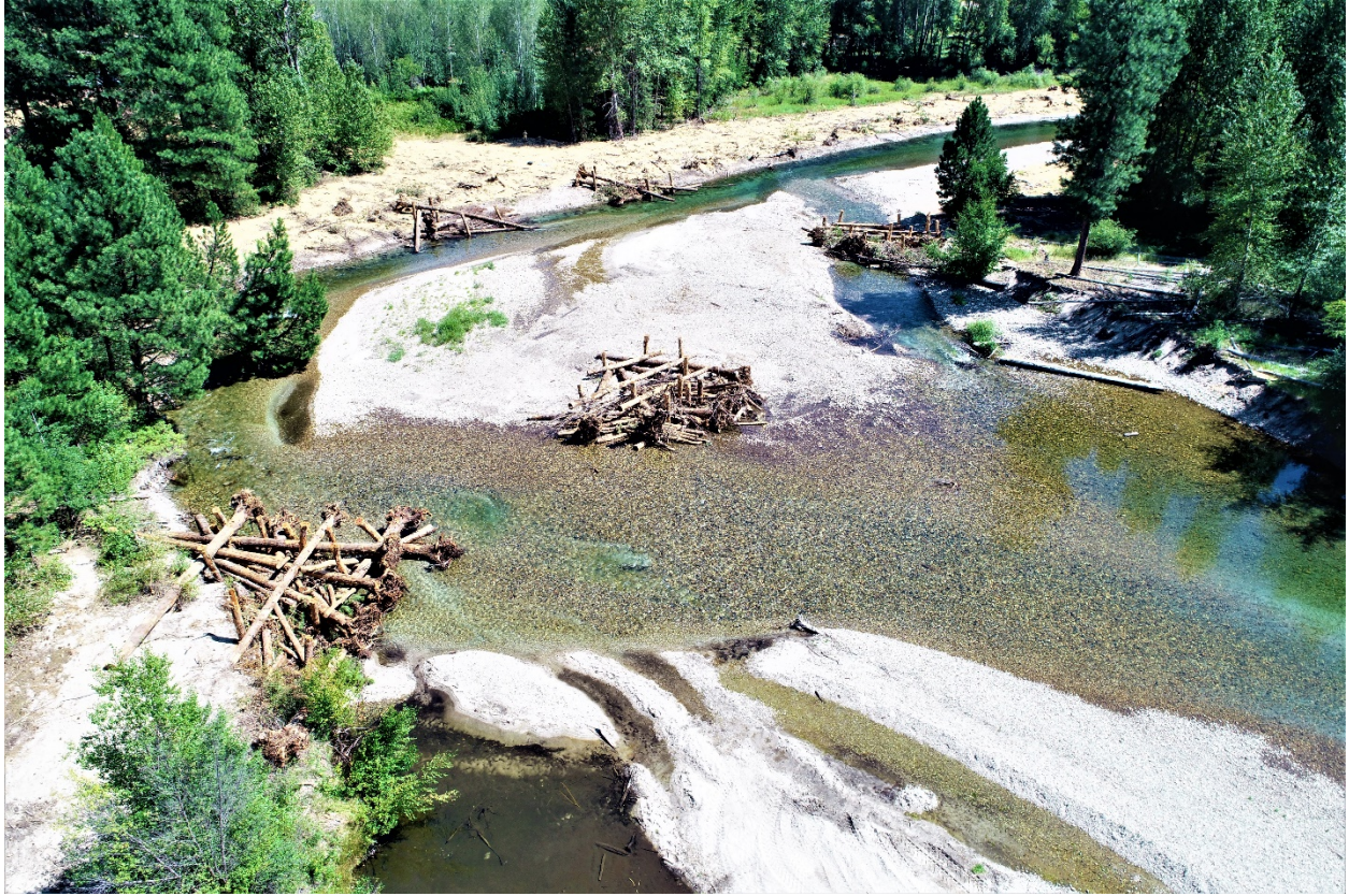
Photograph 29: The levee removal and installation of large wood allow natural river processes to resume along the project length. The natural processes will vastly improve habitat for spawning and rearing salmon and steelhead. (Middle Entiat, Stormy B) (Reclamation/Steve Kolk)
