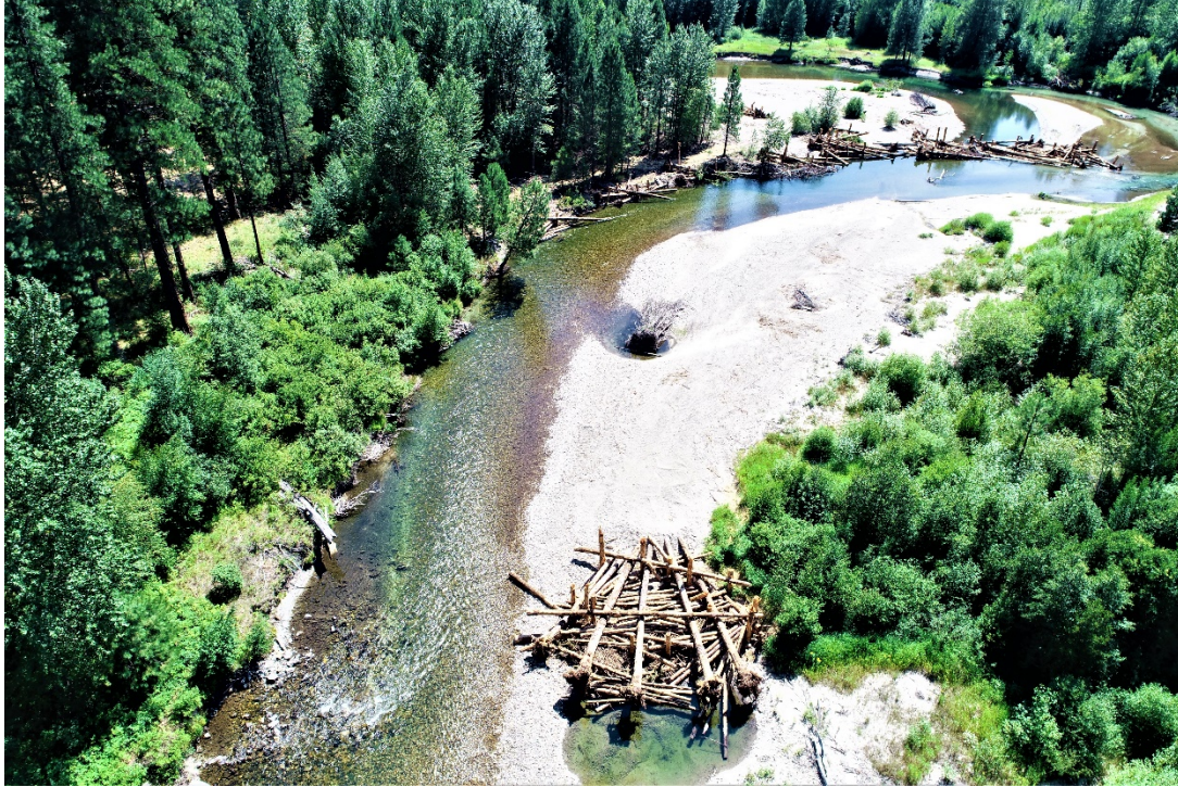
Photograph 25: Large wood was added to the stream to improve fish habitat. The wood structures will provide refuge for juvenile salmonids during high flows. Also, apex structures narrow the channel and force higher flows onto the floodplain and into side channels, which creates beneficial habitat. (Middle Entiat, Stormy B) (Reclamation/Steve Kolk)
