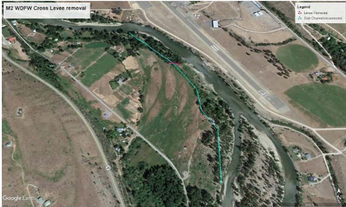
Figure 7: Post-project view shows the levee removed (red line) and side channel reconnected (blue line).
