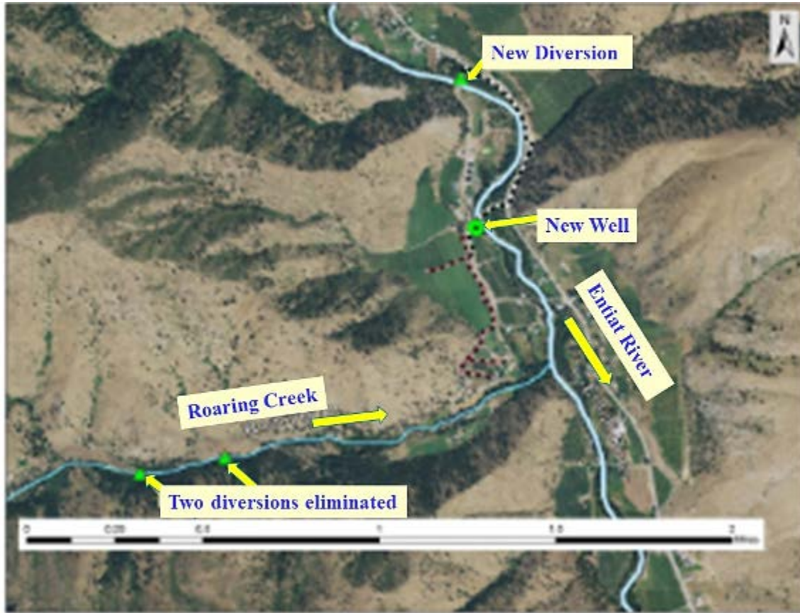
Figure 9: Project map shows the newly created diversion and well. It also shows the two eliminated diversions from Roaring Creek.
