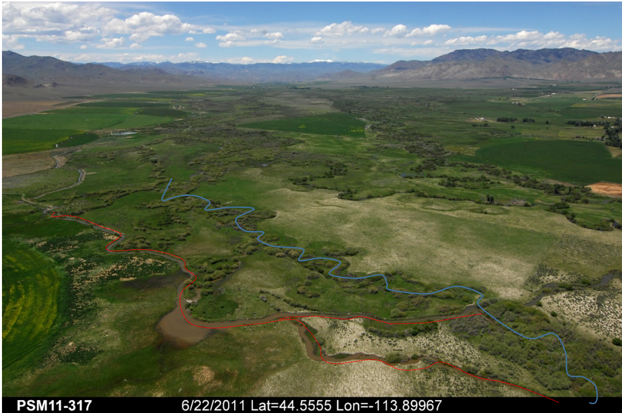
Photograph 27: Aerial view looking downstream along the Pahsimeroi Valley. Flows were taken out of the red marked channel and put into the historic Pahsimeroi River channel marked in blue.
