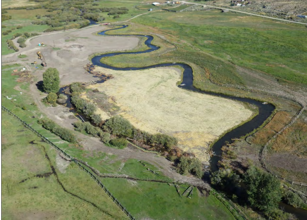
Photograph 11. Upper Lemhi River Side Channel: View of the project area after the old channel was filled, the new channel was constructed, and complexity structures were installed.
