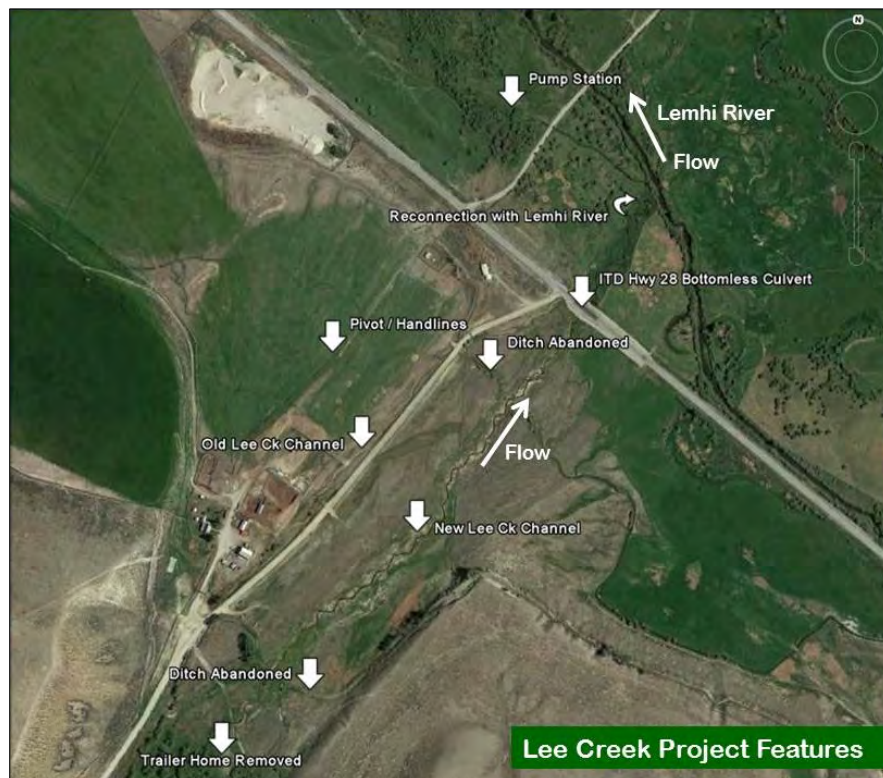
Figure 5. This view shows the many stream habitat improvements in Lee Creek, including the reconnection with the Lemhi River.
