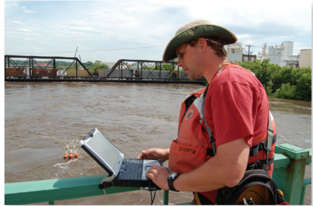
Measuring streamflow on the Cedar River near Cedar Rapids, Iowa. Photograph by Don Becker.
