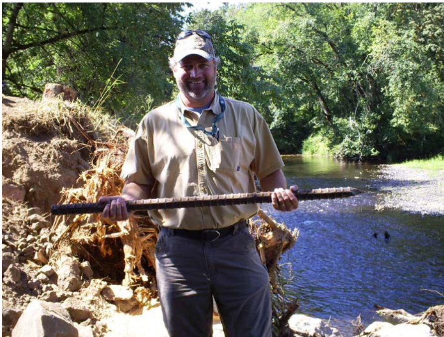
Photograph 12. Steel pin with sharpened end ready for installation into large wood members.
