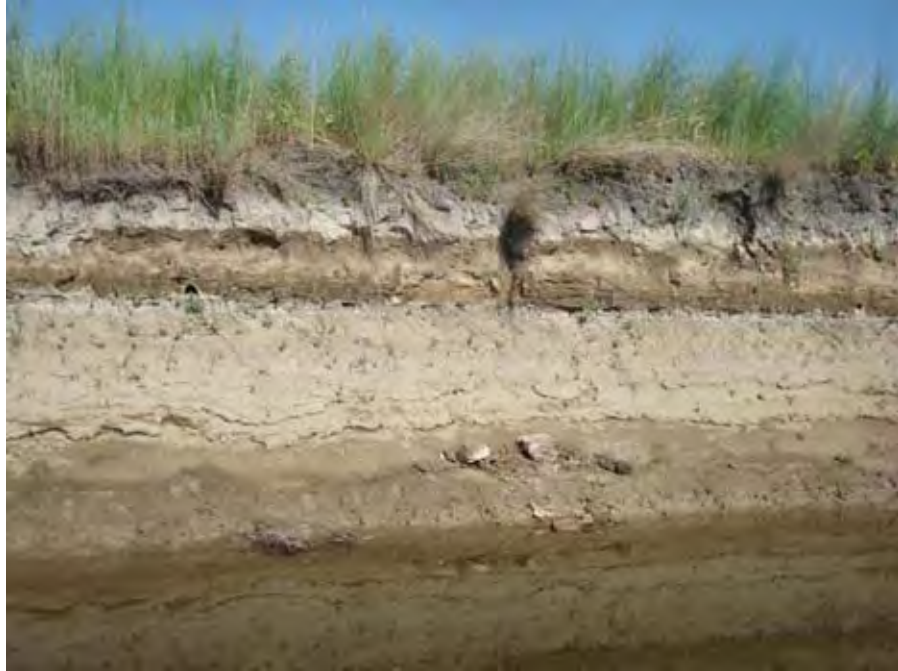
Photograph 215. View from the right bank to the left showing a vertical denuded face and the typical stratigraphy comprised of topsoil over hard, indurated fine-grained material and well-to-poorly indurated silty-clayey sands near river mile 27.86. Reach 2 – Catherine Creek, Grande Ronde Subbasin, Oregon – Bureau of Reclamation Photograph by R. McAfee, July 29, 2010.
