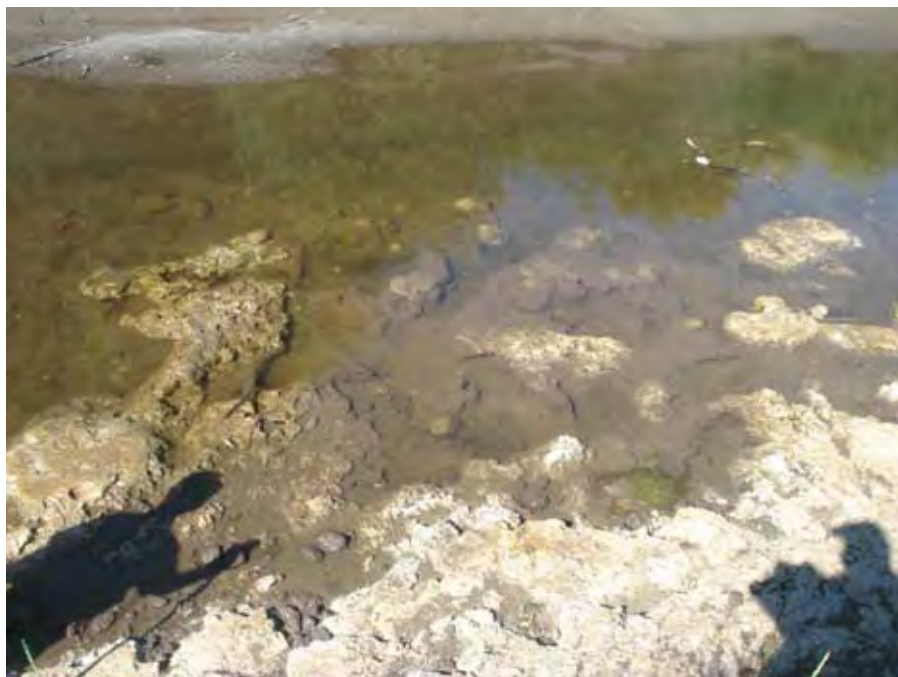
Photograph 91. A close up view of the firm silty material that is erosion resistant, and visible along the toe of the right bank near river mile 33.03. Note the karst-type topography resulting from local ball milling by gravels visible in the lower left of the photograph. Reach 2 – Catherine Creek, Grande Ronde Subbasin, Oregon – Bureau of Reclamation Photograph by R. McAfee, August 1, 2010.
