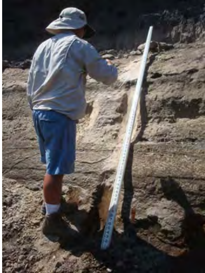
Photograph 259. View of fine-grained alluvial sediments (tan dense silt) exposed on the left (west) bank of Catherine Creek near river mile 22.72. Reach 2 – Catherine Creek, Grande Ronde Subbasin, Oregon – Bureau of Reclamation Photograph by D. Stelma, July 30, 2010.
