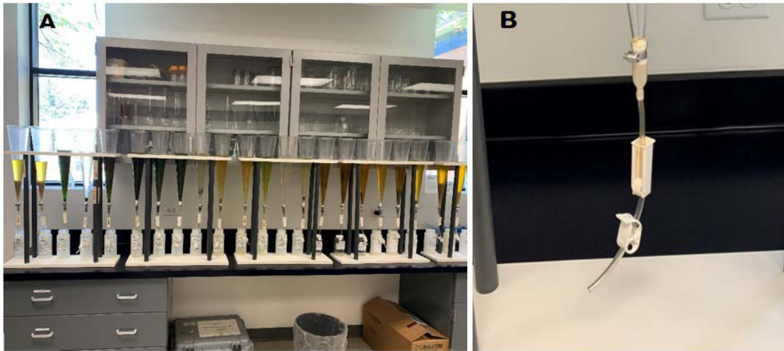
Figure 1: A. Cones are set up with samples. B. Close-up image of the closed roller clamp and the secondary clamp in place on the tubing.
