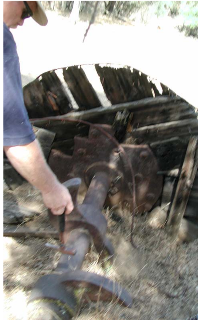
Above: Lift wheel for two-stamp mill (wood construction is unusual); near cabin in Sect.8, R22E, T10S, approximate elevation 860'; inundated by 900' pool contour or greater, RM274 dams site; inundated by any configuration of RM279 dams site (mid-afternoon). (P190091.JPG)
