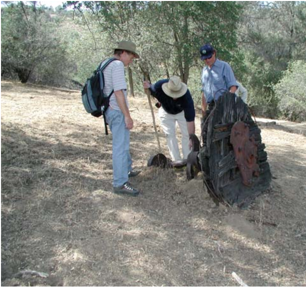
Above: Closer view of MWH team examining lift wheel for two-stamp mill (wood construction is unusual); near cabin in Sect.8, R22E, T10S, approximate elevation 860'; inundated by 900' pool contour or greater, RM274 dams site; inundated by any configuration of RM279 dams site (mid-afternoon). (P190090.JPG)
