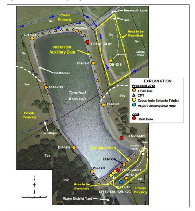
Figure 2: Locations of Geologic Explorations of Terminal Reservoir
